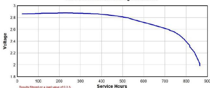
Low Load Pulse Test 300mA Pulse with 2mA Background to 1.8V
